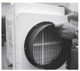
**Step 2:** Using T25 Torx screws, attach the duct plate with collar to the dehumidifier. Attach the top two screws and work down. Do not over tighten the screws.
