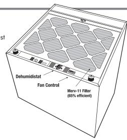
The dehumidifier will run continuously until the relative humidity (RH) is reduced to the humidity control setting. Setting the humidity control to lower RH levels will NOT increase the unit's dehumidification rate, it will simply run longer to reduce the area's RH to the setting.
