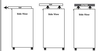
**Step 2 -** Insert the new filter by gently placing it back into the top of the unit. Be sure the arrows on the filter are pointing down towards the unit. Reinstall the top cover by sliding the back in first, then the front. Then slide it all the way back until it is securely into place.
