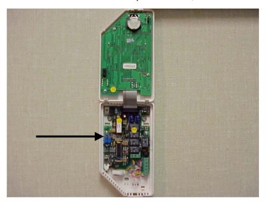
3. To calibrate humidity, use only the left trimmer (R9). Turning clockwise will increase humidity. Only calibrate to an accurate meter!
