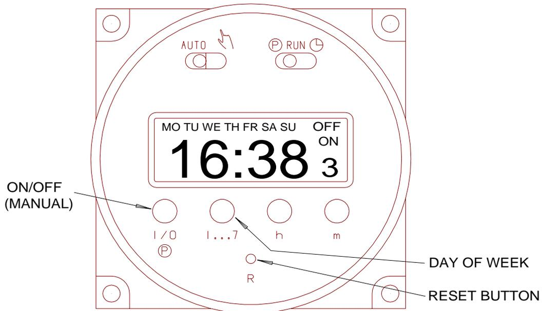
the right) and pressing the **1...7** (DAY), **h** (HOUR), and **m** (MINUTE) buttons. Remember that this timer operates on a 24-hour (military time) clock.
