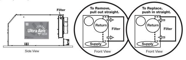
**Step 3:** Insert filter door into bottom tab. Push latch down and swing door shut. Once the door is shut, release the latch.
