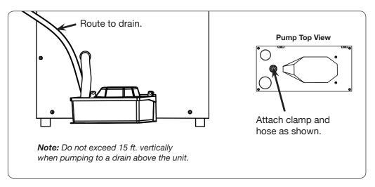
Step 3: Plug the condensate pump cord and dehumidifier cord into an outlet that is protected with a GFCI device on its circuit.
