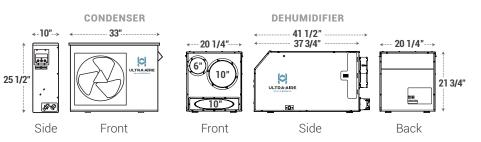
Specifications are subject to change without notice. Power and Performance are based on 80°F/60%RH conditions. Pints / gallons are per day. Sizing is based on 10 foot ceiling height. Unit dimensions and weight are with collars on.
