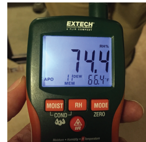
Conditions inside apartment were 74% RH and 66°F.
