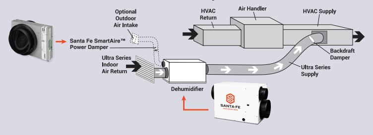
The SmartAire™ Power Damper and any of the Ultra Series dehumidifiers can be wired independently of a home's air handling system.
