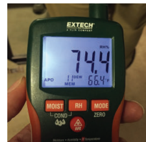
Conditions inside apartment were 74% RH and 66°F.
